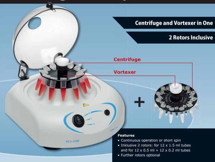
Combined centrifuge/vortex mixer for microtubes and 0.2 ml strips. For independent centrifuge and vortex mixing, or mixing of an individual tube concurrently with spinning of multiple tubes. The vortex cup, located at the top of the central shaft, emerges through an opening in the closed lid. In spin-mix-spin applications, the Combispin can be used with very low reagent volumes.
